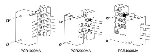
6 Attach a crimping terminal to the switchboard end of the power cord.
