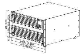
When mounting on a millimeter rack (Bracket model: KRB300)
