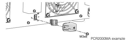
Use the screws to secure the wires in place.
