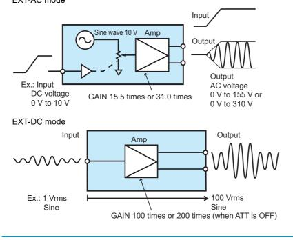
**CAUTION** When the product is being controlled using external analog signals, voltage limits cannot be set. Applying an excessive external voltage by mistake can damage the load.
