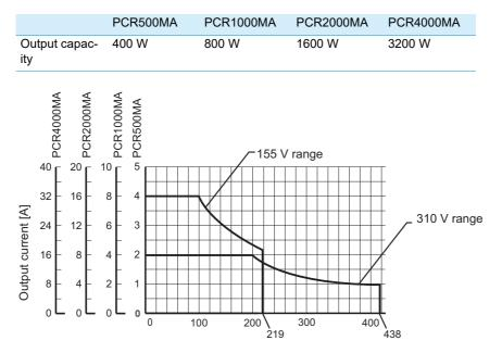
If you use the product with a current that exceeds the rated DC output current, the protection functions will be activated, which may cause the output voltage to drop or turn off the output.
