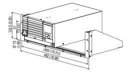
When mounting on a millimeter rack (Bracket model: KRA150)
