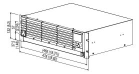
When mounting on a millimeter rack (Bracket model: KRB150-TOS)
