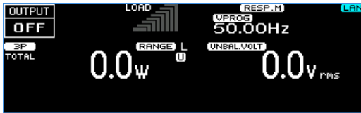
Single-phase display (example of U-phase display)
