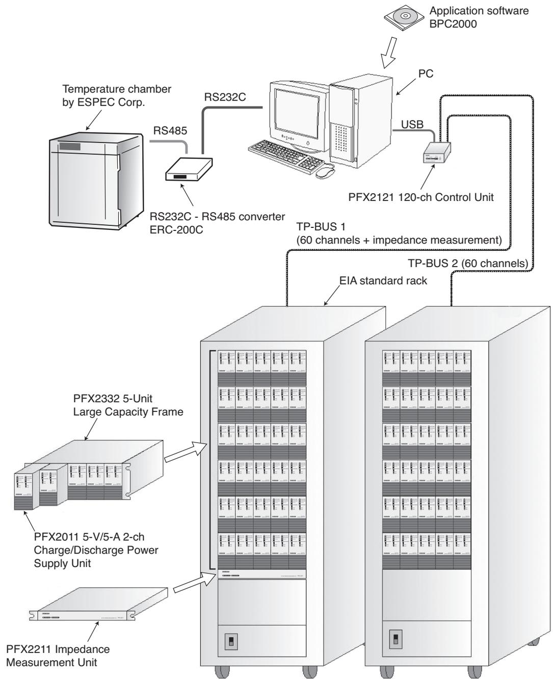
Fig. P-1 120-channel system configuration example
