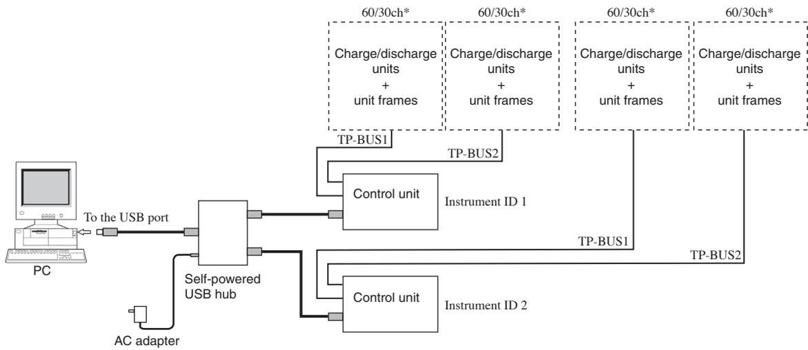
Fig. 1-16 Connection Example of Two Control Units
