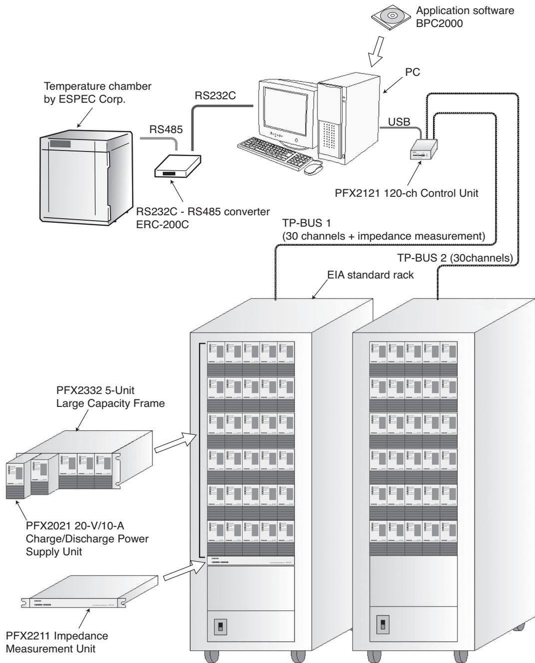
Fig. P-2 60-channel system configuration example
