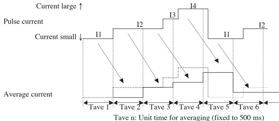
Fig. A-10 Averaging Example 2 of Pulse Current Measurement
