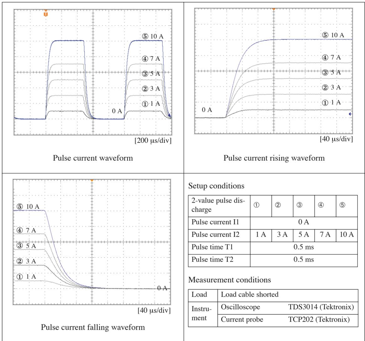
Fig. A-17 PFX2021 Pulse Current Waveform
