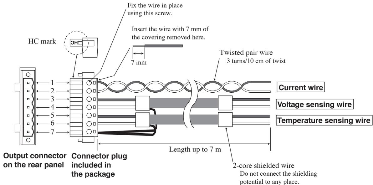
Fig. 2-3 Output Cable Example
