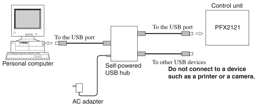
Fig. 1-14 Connection via the USB Hub
