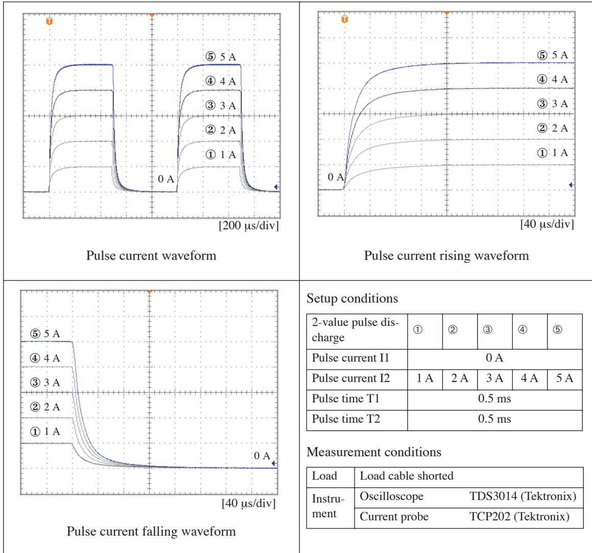
Fig. A-16 PFX2011 Pulse Current Waveform
