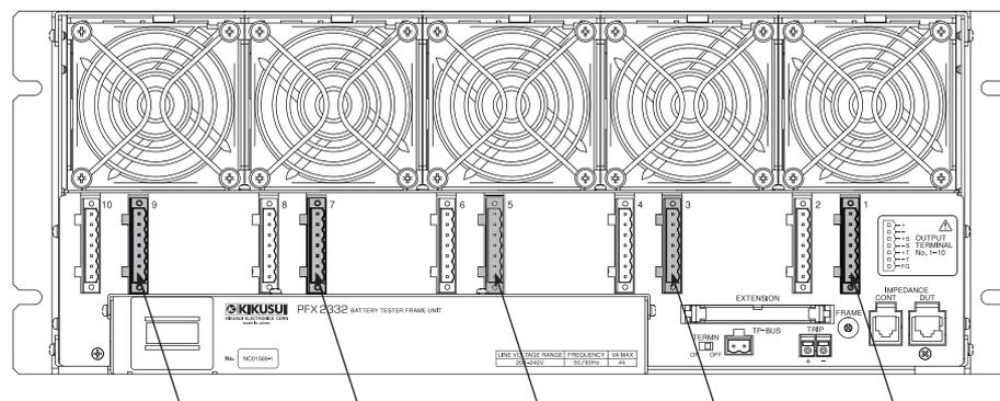
Connect the output cables to the odd-numbered output connectors.
