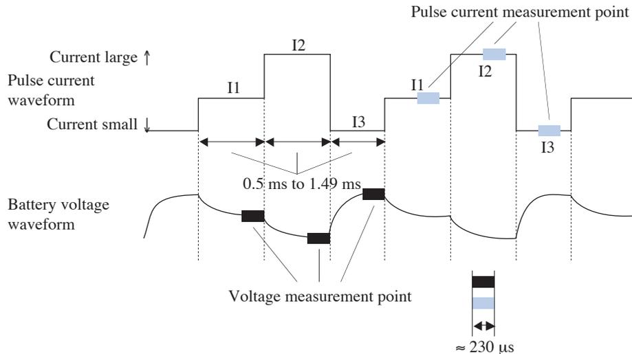
Fig. A-6 Example 2 during Pulse Charge (when the pulse time is less than 1.5 ms)
